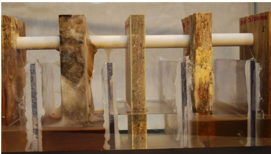
Figure 2: Test samples immersed in water. Plexiglas dividers prevent water movement between samples
