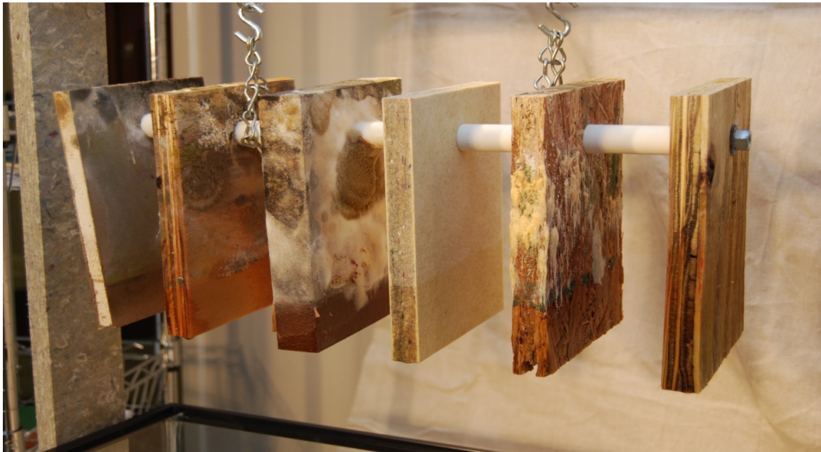
Figure 3: Test samples after 30 days in testing tank. Note mold growth on all the boards except Nyloboard (fourth from left)
